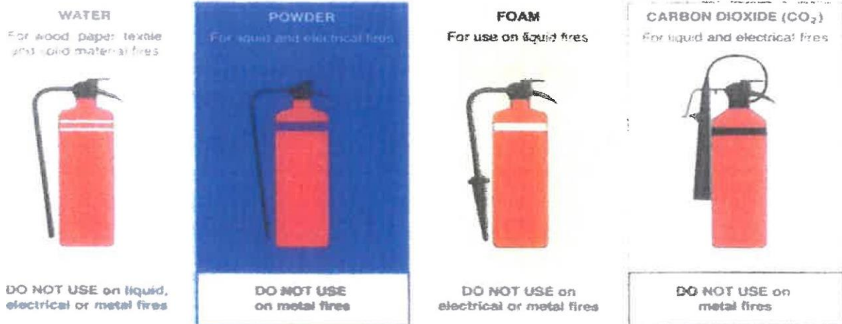
Main types of portable extinguishers, their uses and colour coding
